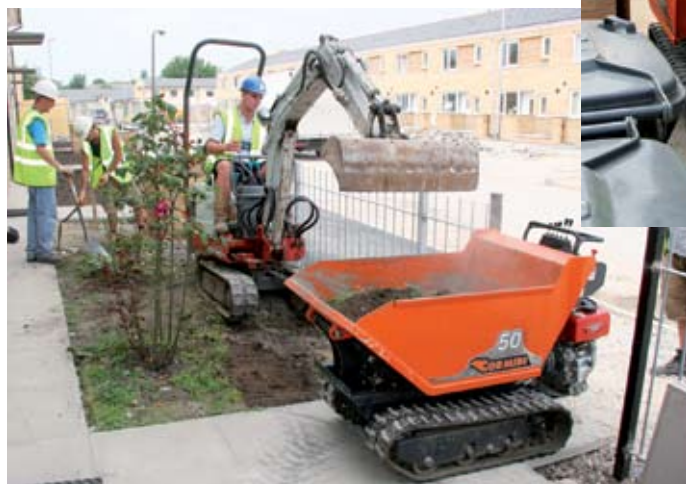
This 6.50 High-Tip from KB Plant Hire has been successfully used by Roots & Shoots to access front and rear gardens during landscaping work in Manchester.
