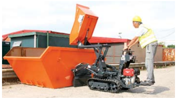
The use of a hydraulically tipped loader bucket and extra travel on the elevation cylinders allows this 10.65 Combi better forward reach at maximum discharge height.
